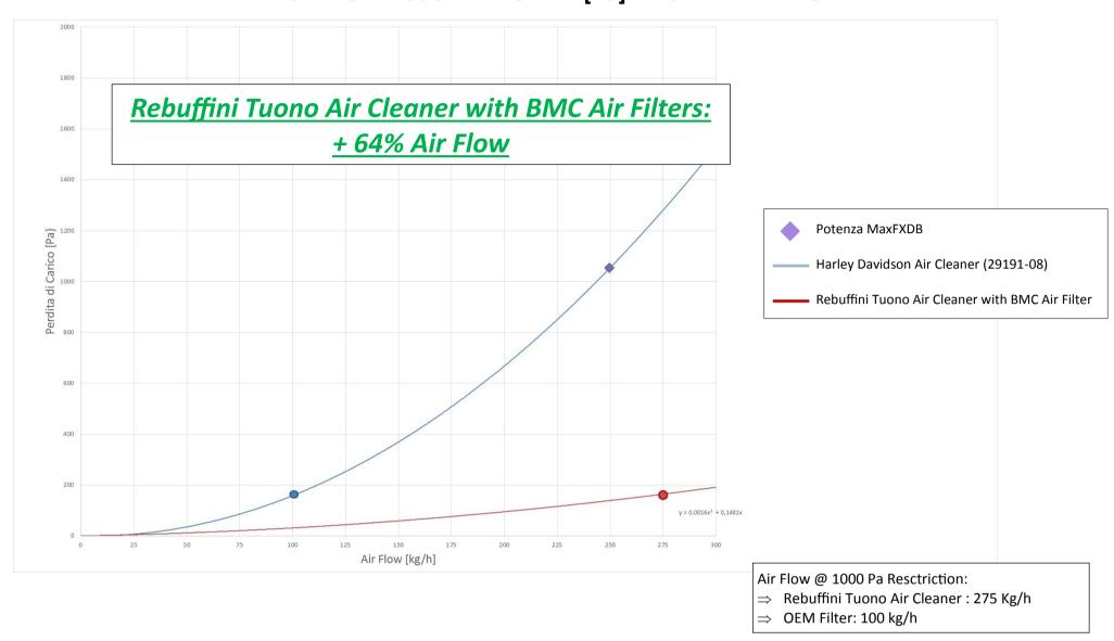
Static Pressure Drop: measure of the loss of Pressure generated by an air filter
