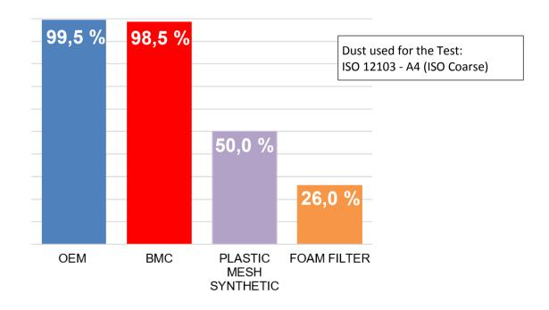
**Filtration Efficiency:** Capacity % of the air filter to block contaminant particles. **Note:** The data results refer to standard filter media materials.
